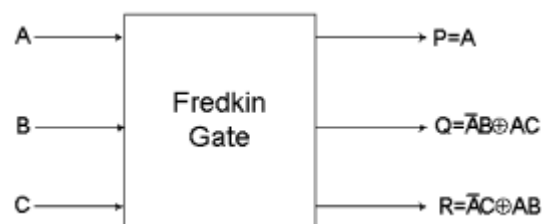
Fig -5: Fredkin Gate Circuit diagram
