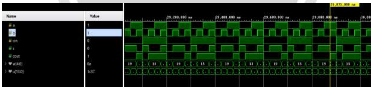
Fig -7: Simulation result of Full Adder
